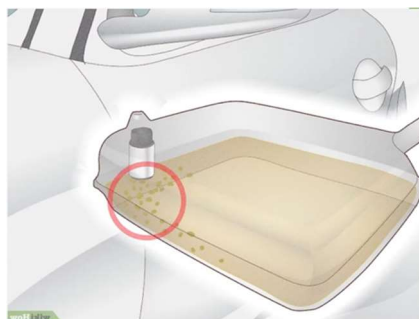
Rusting gas tank
